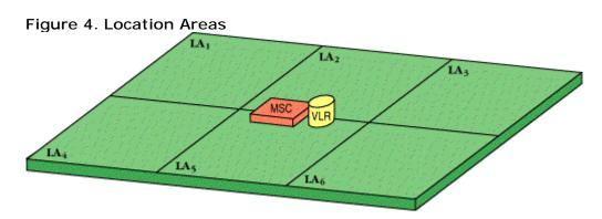
An MSC/VLR service area represents the part of the GSM network that is covered by one MSC and which is reachable, as it is registered in the VLR of the MSC (see *Figure 5*).
