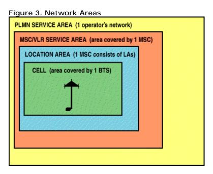
The cell is the area given radio coverage by one base transceiver station. The GSM network identifies each cell via the cell global identity (CGI) number assigned to each cell. The location area is a group of cells. It is the area in which the subscriber is paged. Each LA is served by one or more base station controllers, yet only by a single MSC (see *Figure 4*). Each LA is assigned a location area identity (LAI) number.
